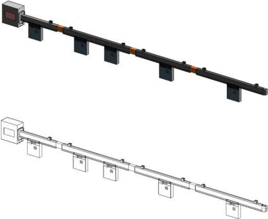
2. PowerWave™ 2 Bus System with **Clearances** turned on.
